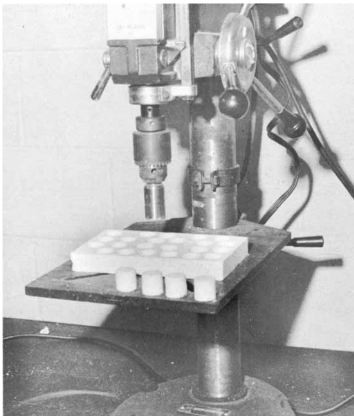
Fig. 2. Preparation of cylindrical samples of urea-formaldehyde foam. Samples were 2.54 cm in diameter.
